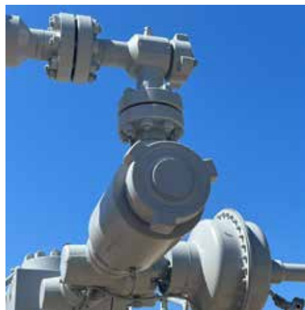
Hundreds of plug catchers have been installed in the field so far
