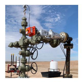
CORTEC produces a full line of compact wellhead plug catchers, which can be installed upstream of the production choke to filter debris, resulting in greater choke performance and reduced production downtime. Our automation team is versed in all common industry requirements, and CORTEC commits to a substantial stocking of actuator options, including Emerson, Rotork, and other OEM options.
