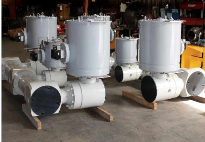
8" x 6.225" API 10K Valves complete with Manifold Sub assemblies
